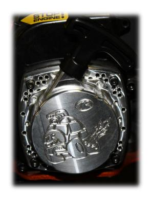
10. Rotate TR Housing assembly till the handle points in the direction you like and use 4pcs. M4x10SocketHeads to secure TR housing, holes in TR housing must line up with threaded holes in adapter plate. The holes in TR adapter plate are every 22.5degrees to offer you several options.
