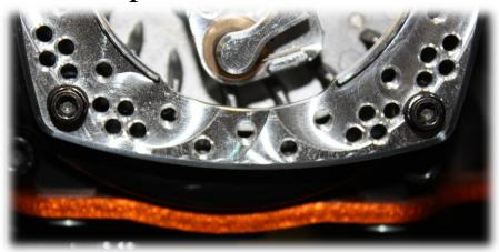
9.Install TR PullStart housing assembly onto adapter plate. Set cog on one of the dogs holding housing at an angle, push down on housing to force dog open then wiggle housing against adapter plate. This might take a little finesse since you need to get the cog between both dogs. The housing will sit flat against the adapter plate when finished.
