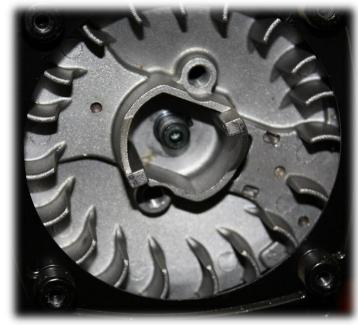
5.Install TurtleRacing Flywheel nut, use some thread lock and tighten with small end of spark plug wrench.
