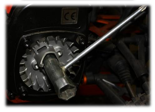
6.Install TR Dog Cage assembly, use thread lock on M5x12 FlatHead. Rotate "cutouts" on dog cage against "ears" on flywheel then tighten M5x12 FlatHead.
