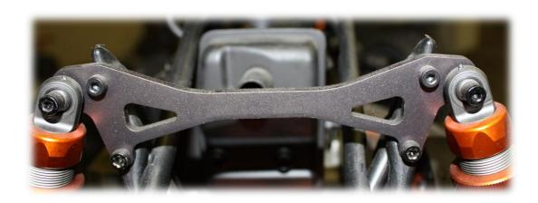
2.Install mount using 2pcs-M4x35 flatheads in the lower holes and 2pcs-M4x25 socketheads in the top holes. The top screws are longer than stock and will go through the stock plastic shock towers. You have 2 options- drill through the plastic with 1/8" (3mm) drill or just drive the screws right through.
