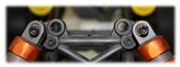
2. Install 2pcs M4x35 Flathead in shock tower. These screws are longer than stock and will go through the plastic shock tower. Either drill through shock tower with a 1/8" (3mm) drill or just drive the screw through the plastic. After you drive screw through, back it out and trim plastic flat with a knife or Dremel, run screws back in and install M4 locknuts.
