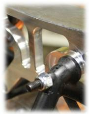
**5.** Reinstall the 2 stock (wood style) screws into lower combo mount (backside).
