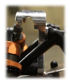
4. Install 2pcs M4x35 Flathead in shock tower. These screws are longer than stock and will go through the plastic shock tower. Either drill through shock tower with a 1/8" (3mm) drill or just drive the screw through the plastic. After you drive screw through, back it out and trim plastic flat with a knife or Dremel, run screws back in and install M4 locknuts.
