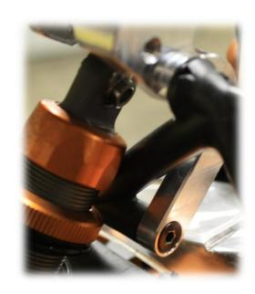
6. Insert shocks into mount, install and tighten M4x30 ButtonHead.
