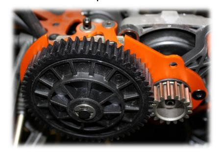
3. Remove 7 screws holding trans plate, gear plate, brake assembly, brake rotors and brake hex.
