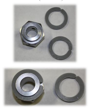
9. Install brake hex onto Baja, plastic ring towards transmission.
