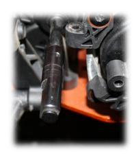
4. Remove 2 screws holding shock tower supports.
