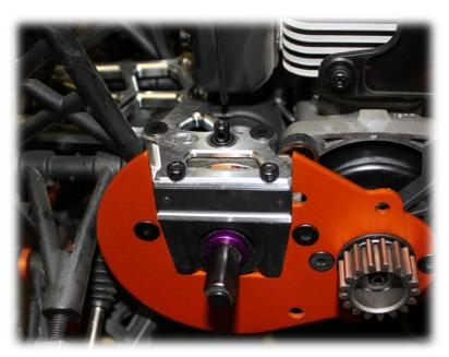
15. Install "purple" spacer, spur gear, gear cover, cage and body/body panels.
